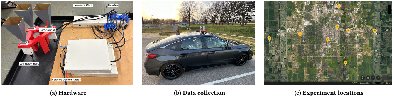
Figure 10: Experimental Setup – We use a 2D array of LNBS to sniff the transmissions of satellites passing overhead at 8 different locations (location labels removed for anonymity)
